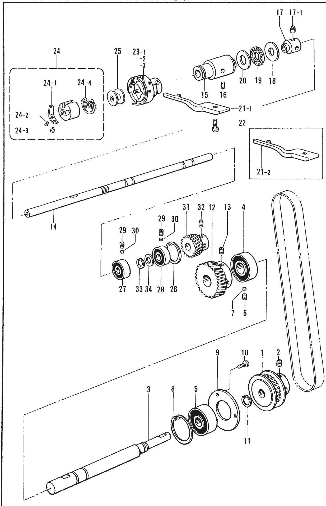
F. カマ関係/Rotary hook mechanism/Greifervorrichtung/
