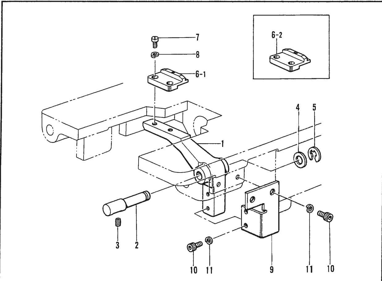
D. 糸切れ感知関係/Thread breakage detector mechanism/Fadenbruchfühler/
