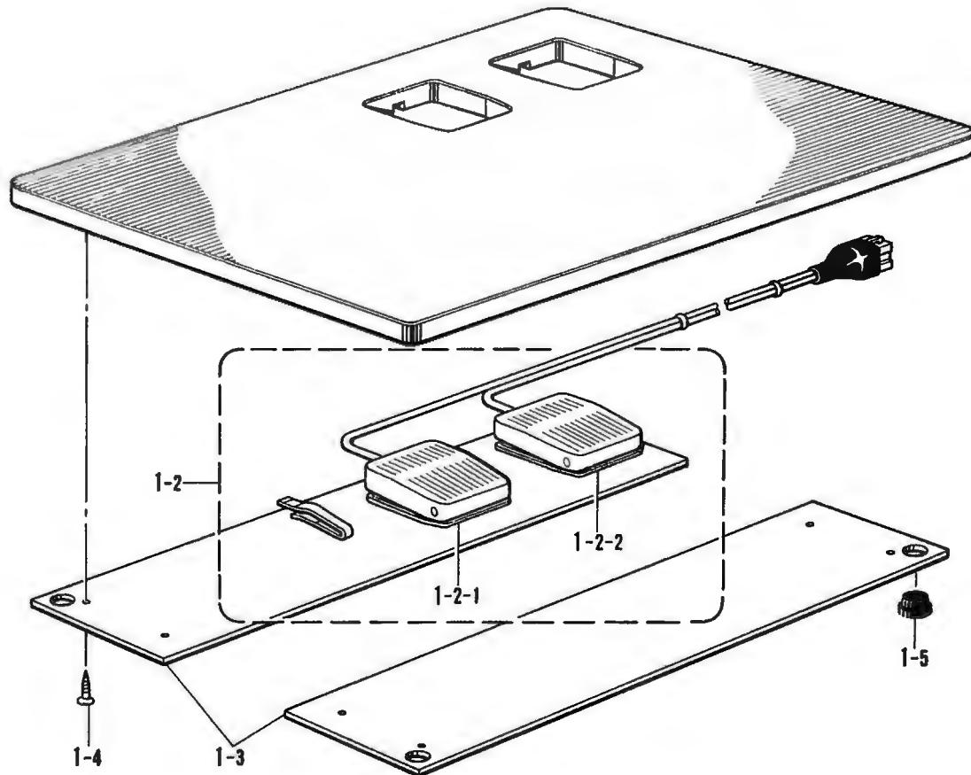
B1. 踏板関係/Foot switch pedal mechanism/Pedal/
