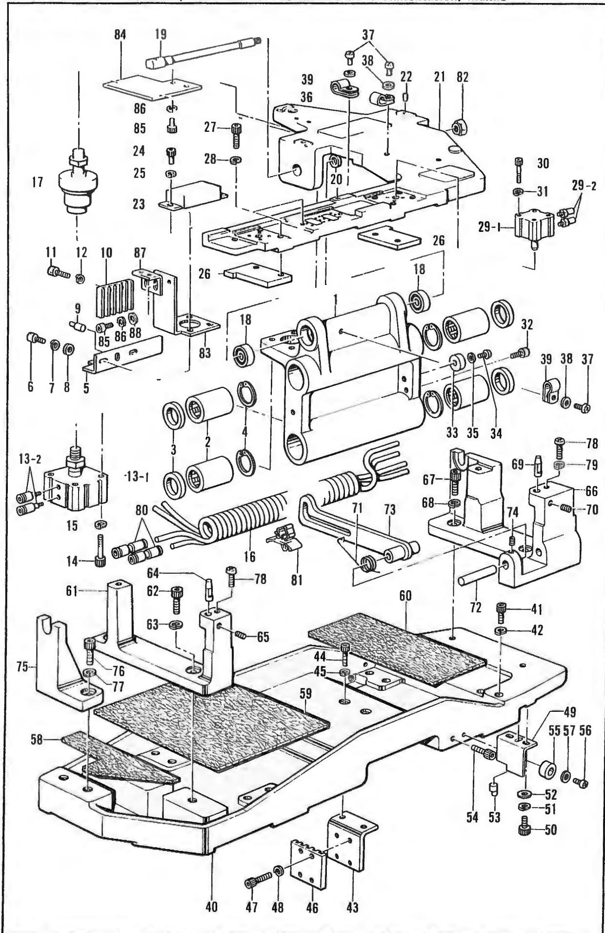
R. 駆動側・送り関係 / Drive, feed mechanism / Transportvorrichtung /
