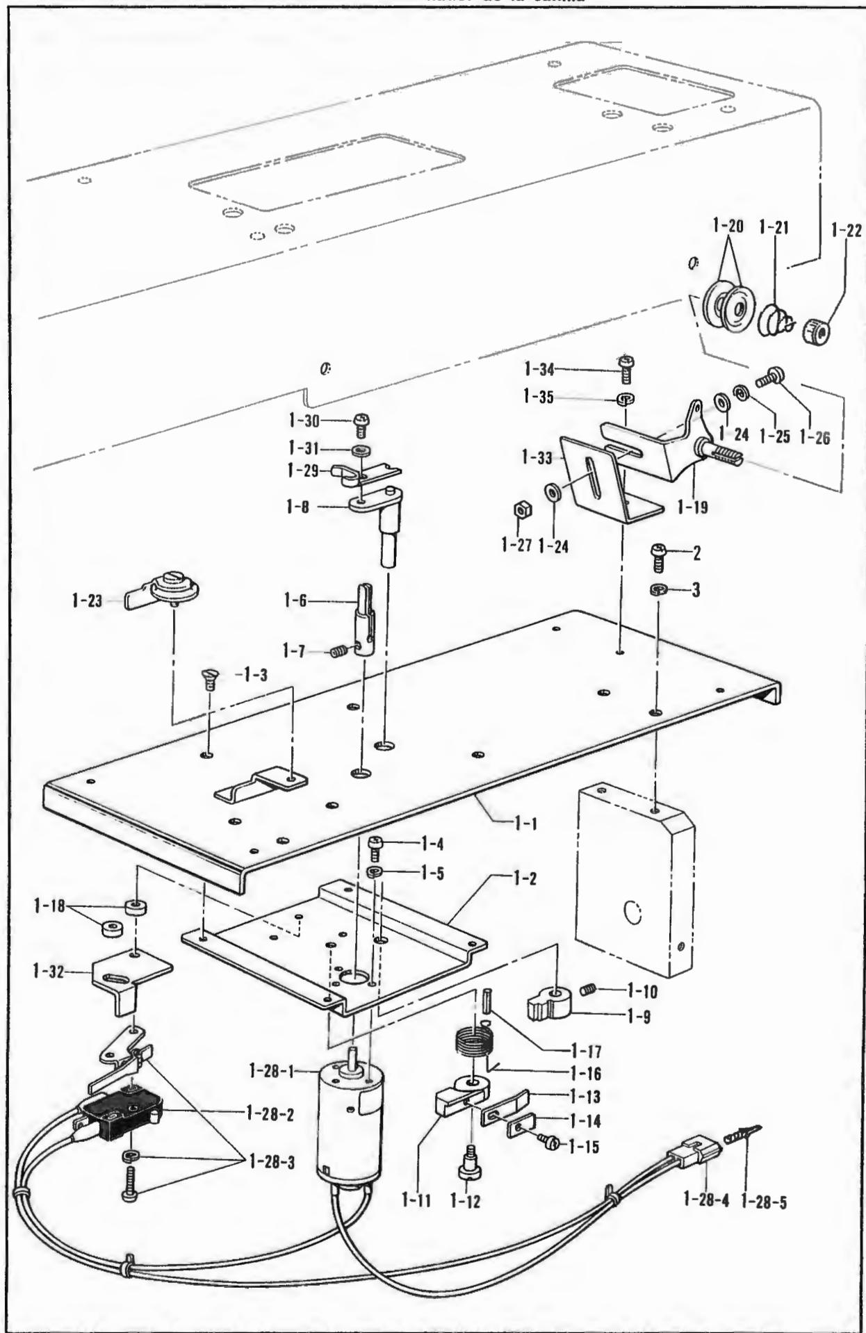
V. 糸巻関係 / Bobbin winder mechanism / Spuler /
